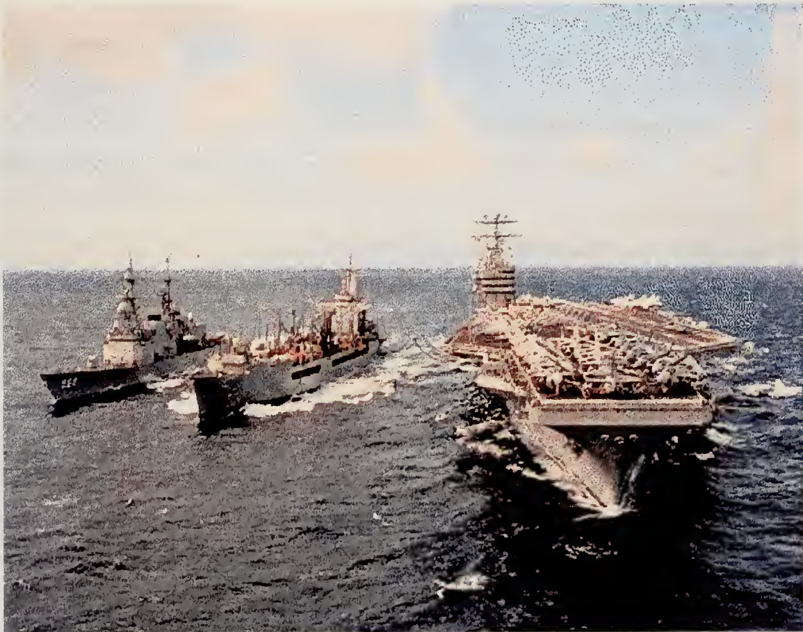
Figure I-1 USS GEORGE WASHINGTON (CVN 73) and USS ARTHUR W. RADFORD (DD 968) performing simultaneous underway replenishment of JP-5 fuel from USS MERRIMACK (AO 179) in support of operation "Joint Endeavor."
